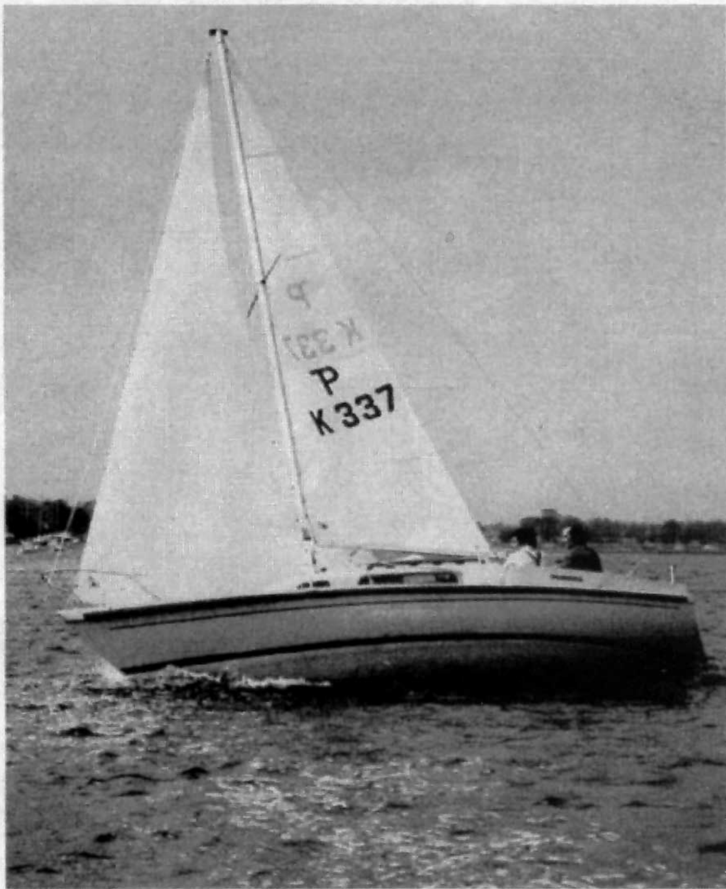
Lacking the exaggerated beam of the modern crop of IOR orientated boats, Pandora International heels quickly to about 15°, at which point she stiffens and becomes reluctant to heel further. Even when the boat is well heeled the helm remains light, and the boat is responsive and well balanced.
